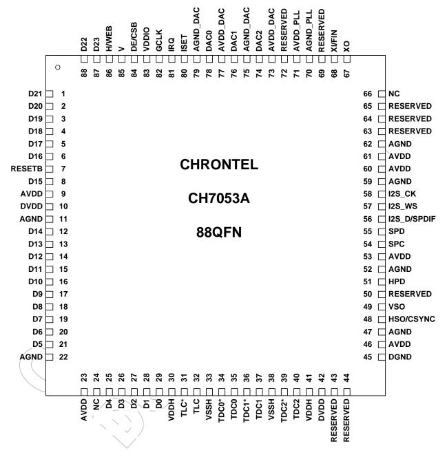
Figure 2: 88 pin QFN Package (Top View)
