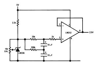
Figure 26. Low Noise Buffered Reference
