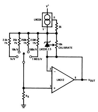
Figure 21. Linear Ohmmeter
