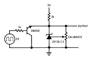
Figure 24. 2.5V Square Wave Calibrator
