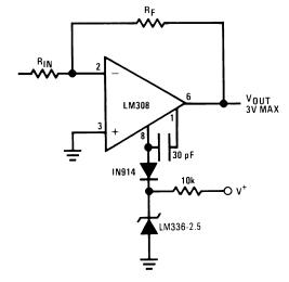
Figure 22. Op Amp with Output Clamped
