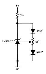
Figure 5. 2.5V Reference with Minimum Temperature Coefficient
