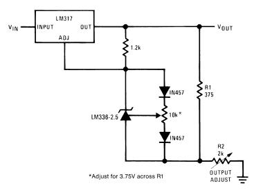
Figure 17. Precision Power Regulator with Low Temperature Coefficient
