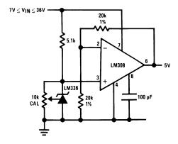
Figure 25. 5V Buffered Reference
