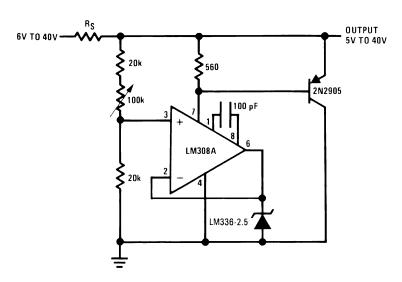
Figure 20. Adjustable Shunt Regulator
