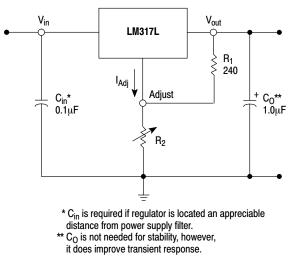
$$V_{out} = 1.25 V \left(1 + \frac{R_2}{R_1}\right) + I_{Adj} R_2$$
