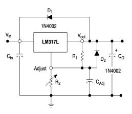
Figure 19. Voltage Regulator with **Protection Diodes**
