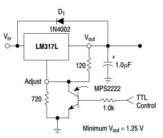
D<sub>1</sub> protects the device during an input short circuit.
