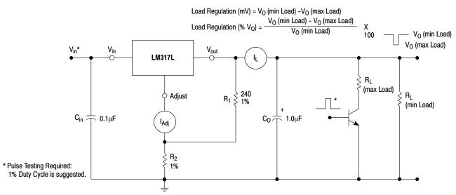
Figure 3. Load Regulation and  $\Delta I_{Adj}$ /Load Test Circuit
