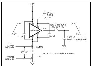
**FIGURE 4-2:** Switching Time Degradation Due to Negative Feedback.
