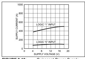
FIGURE 2-10: Quiescent Power Supply Voltage vs. Supply Current.
