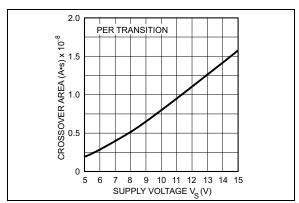
FIGURE 2-15: Crossover Area vs. Supply Voltage.
