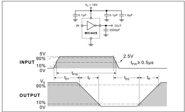
FIGURE 1-1: Inverting Driver Switching Time.
