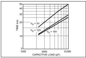
FIGURE 2-5: Fall Time vs. Capacitive Load.
