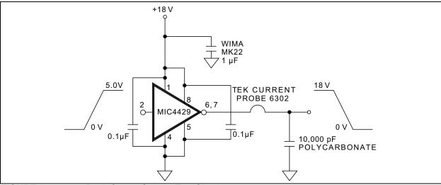
FIGURE 4-3: Peak Output Current Test Circuit.
