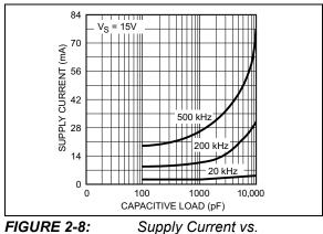
FIGURE 2-8: Capacitive Load.
