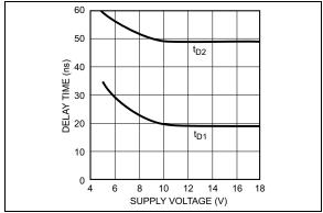
FIGURE 2-6: Delay Time vs. Supply Voltage.
