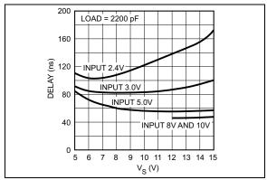
FIGURE 2-14: Effect of Input Amplitude on Propagation Delay.
