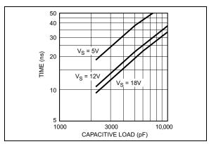
FIGURE 2-4: Rise Time vs. Capacitive Load.
