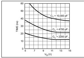
**FIGURE 2-1:** Rise Time vs. Supply Voltage.
