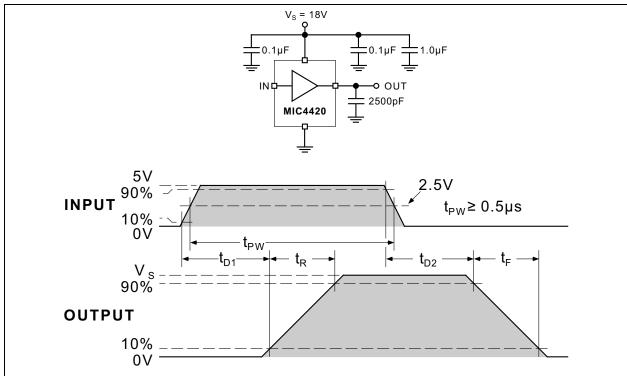
FIGURE 1-2: Noninverting Driver Switching Time.
