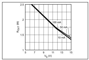
FIGURE 2-13: Low-State Output Resistance.
