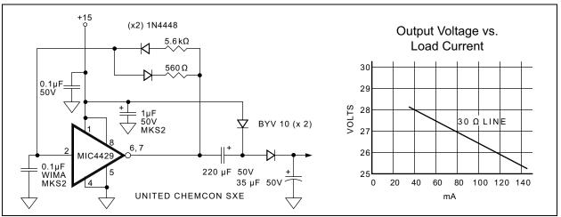
FIGURE 4-1: Self-Contained Voltage Doubler.
