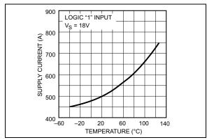
**FIGURE 2-11:** Quiescent Power Supply Current vs. Temperature.
