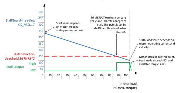
Figure 11.1 Function principle of StallGuard4
