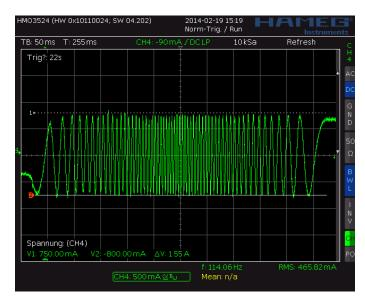
Figure 6.3 Scope shot: good setting for PWM\_REG
