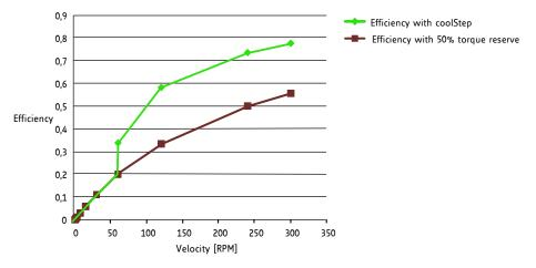
Figure 1.3 Energy efficiency with coolStep (example)
