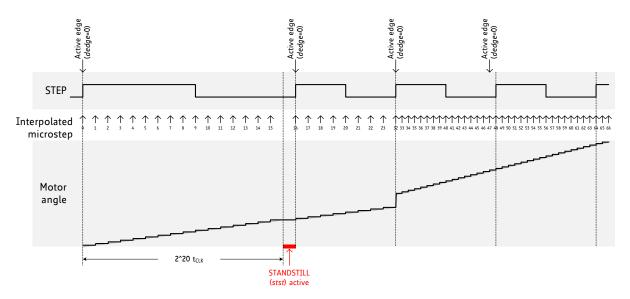
Figure 13.2 MicroPlyer microstep interpolation with rising STEP frequency (Example: 16 to 256)
