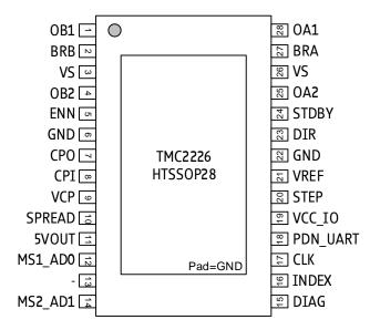
Figure 2.1 TMC2226 Pinning Top View - type: HTSSOP 28, 9.7x6.4mm<sup>2</sup> over pins, 0.65mm pitch
