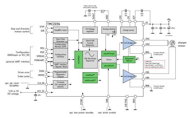
Figure 3.2 Application circuit using RDSon based sensing
