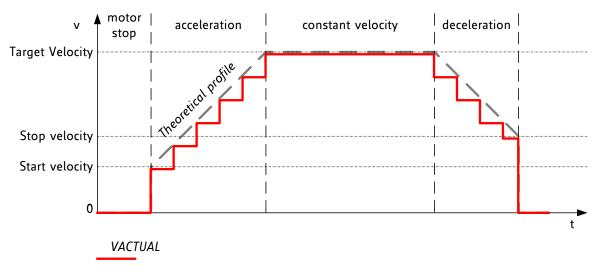
Figure 14.1 Software generated motion profile
