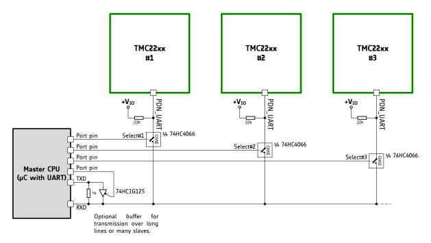
Figure 4.2 Addressing multiple TMC2226 via single wire interface using analog switches
