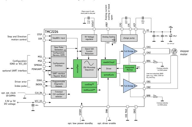
Figure 1.1 TMC2226 basic application block diagram
