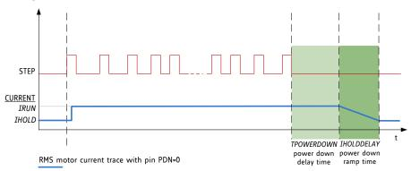
Figure 1.4 Automatic Motor Current Power Down
