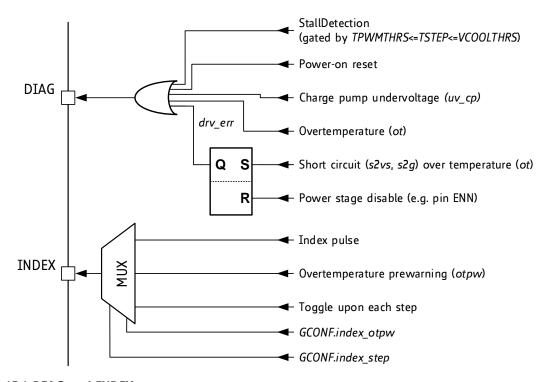
Figure 15.1 DIAG and INDEX outputs
