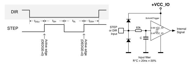
Figure 13.1 STEP and DIR timing, Input pin filter
