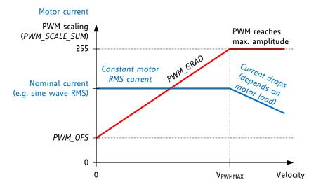
Figure 6.6 Velocity based PWM scaling (pwm\_autoscale=0)
