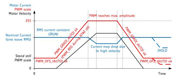
Figure 6.5 Successfully determined PWM\_GRAD(\_AUTO) and PWM\_OFS(\_AUTO)
