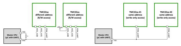
Figure 4.1 Attaching the TMC2226 to a microcontroller UART
