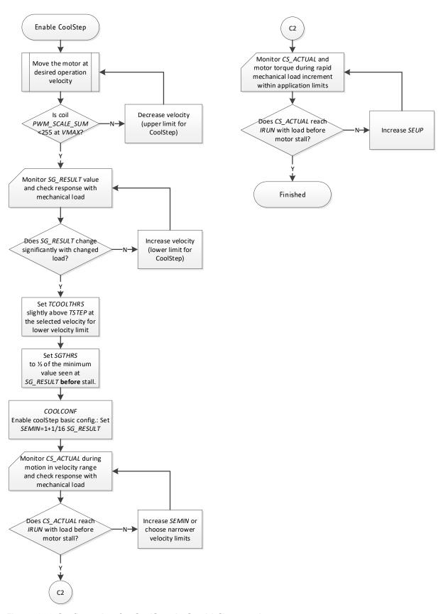
Figure 16.3 Configuration for CoolStep in StealthChop mode
