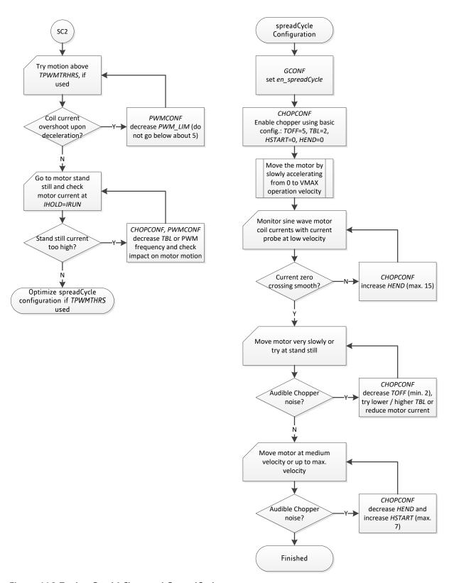
Figure 16.2 Tuning StealthChop and SpreadCycle
