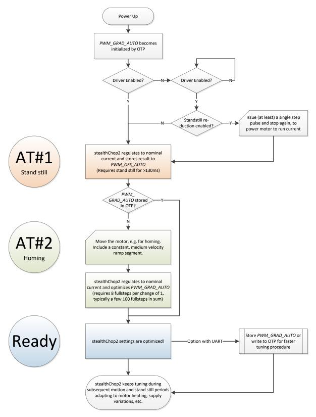
Figure 6.2 StealthChop2 automatic tuning procedure
