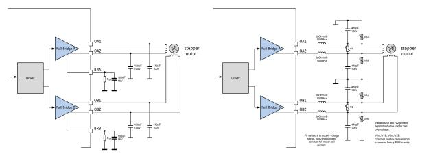
Figure 3.4 Simple ESD enhancement and more elaborate motor output protection
